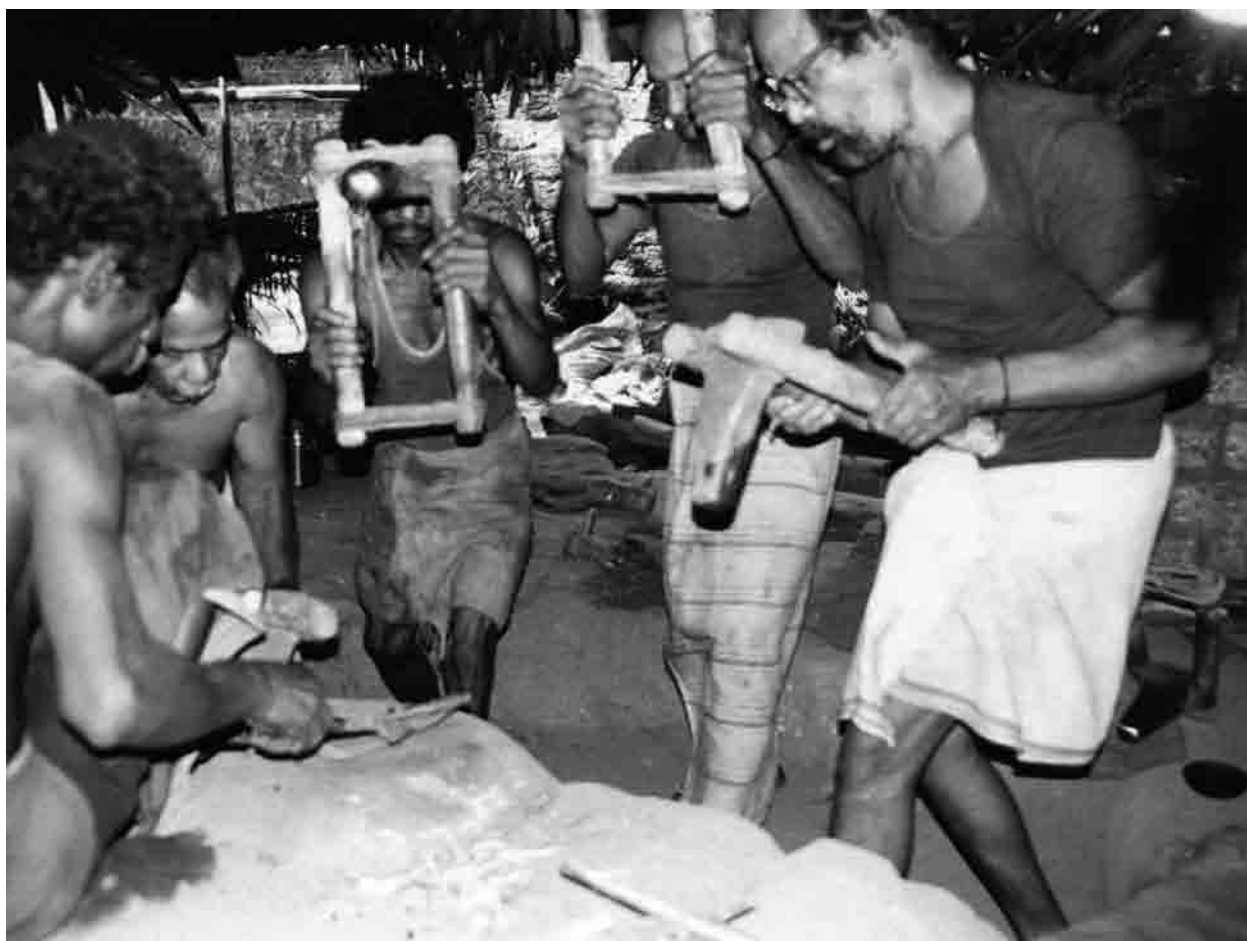
Fig.4. Wrought hammering of heated ingot of high-tin beta bronze (23% tin) in consecutive cycles in Palakkad, Kerala by hammering of red hot ingot in temperature range of formation of plastic beta phase (650-750°C) (Sharada Srinivasan).
