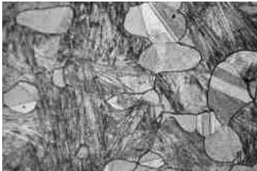
Fig.6. Alpha plus beta martensite structure of hot forged and quenched beta bronze, at around 650 degrees. The annealing twins in the islands of alpha phase indicate a high degree of hot forging (Sharada Srinivasan).
