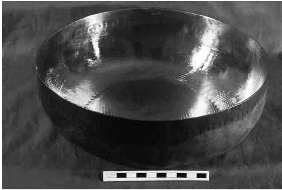
Fig.5. Modern high-tin beta bronze vessel from Payangadi (22.5%). A flat ingot of about 15cm diameter was forged out into a large concave bowl of about 30cm diameter (Sharada Srinivasan).
