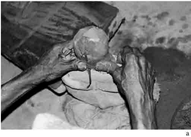
Fig.8. a: Crucible-cum-mould being sealed with cloth dipped in silt and straw/cotton wick. b: Inverted crucible-cum-mould, with the red hot mouth being packed with mud. (Sharada Srinivasan)
